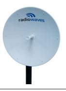
The SP Standard Performance 5W Series by RadioWaves offers a cost effective, dual polarized, 3ft parabolic antenna engineered to deliver reliable radio links with a stable 33 dBi gain from 4.9 to 6 GHz.
