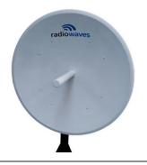
The SP Standard Performance 5W Series by RadioWaves offers a cost effective, dual polarized, 4ft parabolic antenna engineered to deliver reliable radio links with a stable 35.4 dBi gain from 4.9 to 6 GHz.
