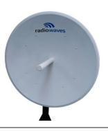
The SP Standard Performance 3.5GHz Series by RadioWaves offers a cost effective, dual polarized, 4ft parabolic antenna engineered to deliver reliable radio links with a stable 30.6 dBi gain from 3.3 to 4.2 GHz. Designed for CBRS, C-band, private LTE, and world-wide CBRS applications, RadioWaves field-proven pre-assembled SP antennas and robust pole-mounts ensure "set and forget" installation with minimal post-installation maintenance. If it's rugged, it must be RadioWaves!
