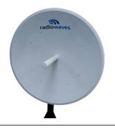
The SP Standard Performance 3.5GHz Series by RadioWaves offers a cost effective, single polarized, 4ft parabolic antenna engineered to deliver reliable radio links with a stable 30.6 dBi gain from 3.3 to 4.2 GHz. Designed for CBRS, C-band, private LTE, and world-wide CBRS applications, RadioWaves field proven preassembled SP antennas and robust pole mounts ensure "set and forget" installation with minimal post installation maintenance. If it's rugged, it must be RadioWaves!
