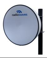
The HP High Performance 5W Series by RadioWaves offers a cost effective, dual polarized, 3 ft parabolic antenna engineered to deliver reliable radio links with a stable 32.8 dBi gain and enhanced protection from link interference over 4.9 to 6 GHz.
