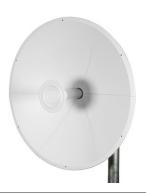
The Radiowaves CCPD2-6RSP collapsible parabolic antenna is designed for point-to-point communications by directing waves to the receiver at its focal point via a parabolic reflector. This antenna has a 30 dBi high gain. Our point to point antenna has a 50 Ohms impedance and is highly directional, which means it receives greater power in a specific direction.
