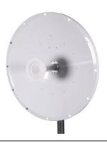
The Radiowaves CSPD2-6RSP parabolic antenna is designed for point-to-point communications by directing waves to the receiver at its focal point via a parabolic reflector. This antenna has a 30 dBi high gain. Our point to point antenna has a 50 Ohms impedance and is highly directional, which means it receives greater power in a specific direction.
