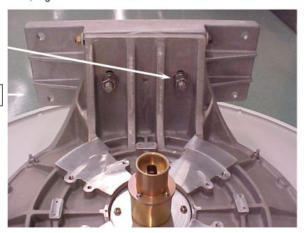
**Feed Orientation**: If Plane Feed has been ordered, the factory default is Vertical Polarization. Refer to supplemental instructions to adjust the feed to horizontal polarization.
