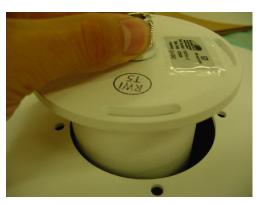
For Vertical Polarization, secure the feed with the arrow as shown
