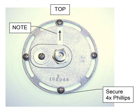
For Horizontal Polarization, secure the feed with the arrow as shown
