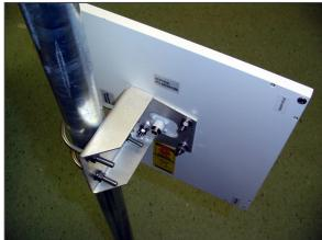
Twist antenna on pole to adjust azimuth
