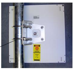
**3. Elevation Adjustment:** (SINGLE AND DUAL POLARITY) Loosen u-bolt nuts slightly so the antenna is able to move. Adjust Elevation as shown:
